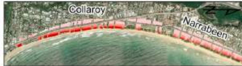
Erosion risk at a Sydney Beach by 2100; SSP5-8.5
